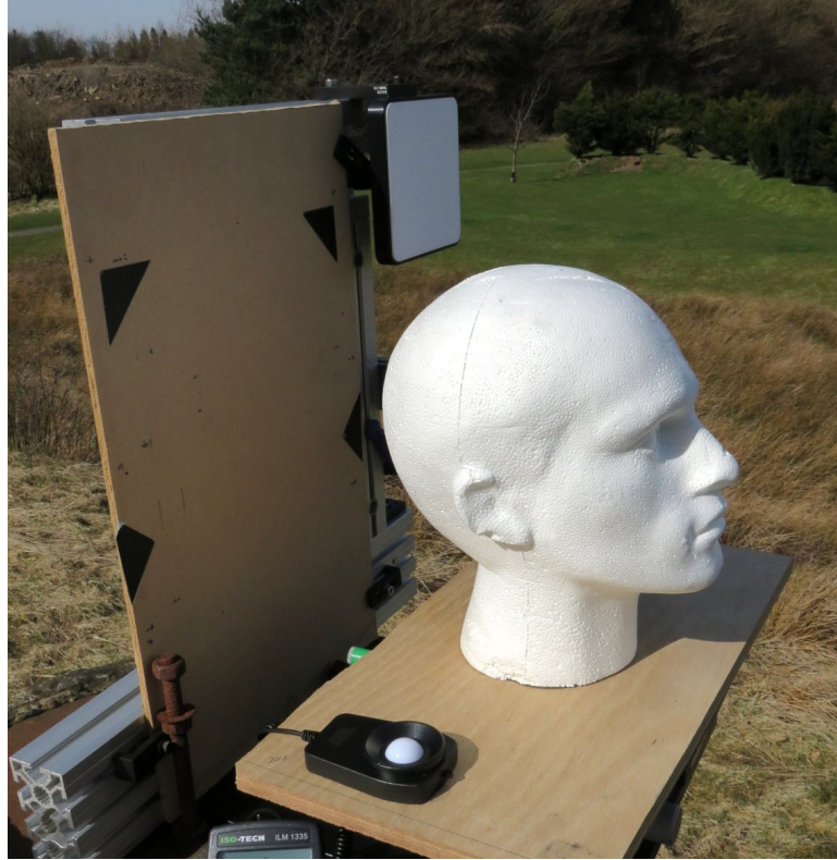
Figure 5.4: Image of the setup used for acquiring single-spectral LIDAR images. The imaged object provides a realistic shape for evaluating the decoding algorithm.
